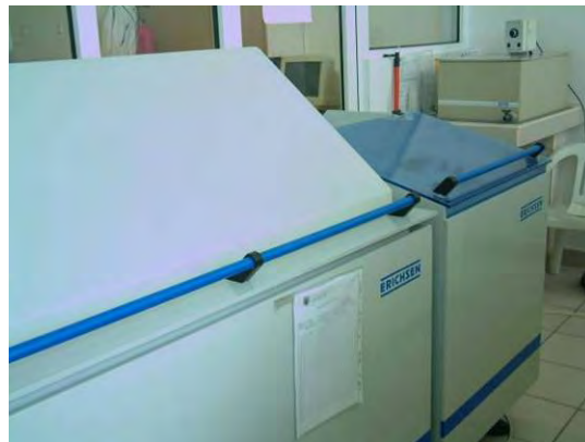
Fig. 1. Installation of oxidant nitrocarburizing Fig. 2. The salt fog chamber used for the experiments
