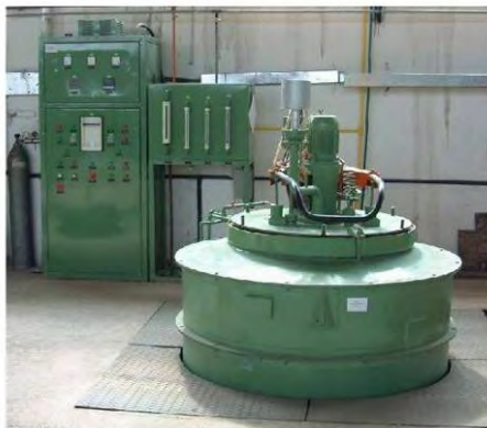
Fig. 1. Installation of oxidant nitrocarburizing Fig. 2. The salt fog chamber used for the experiments
