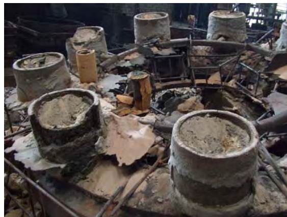
Fig.4. Casting technology by using exothermic heads
