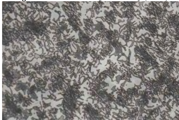
Fig. 3. Microstructure of FeAlMn alloy (X160)
