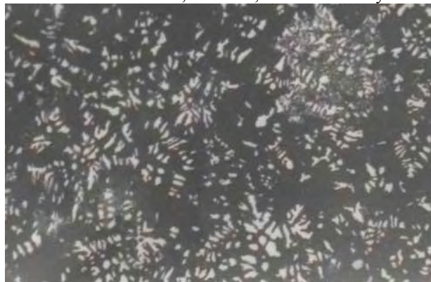
Fig. 2. Microstructure of FeAl alloy (X160)
