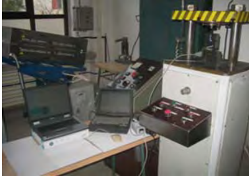
Fig.2. The 20 tones force hydraulic press and the equipment for force measuring
