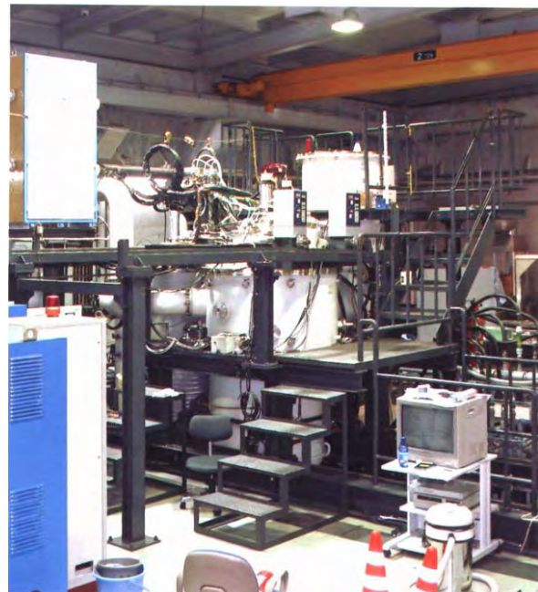
Fig. 10. 500 kW electron beam unit for silicon remelting
