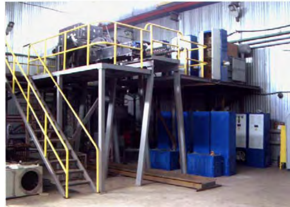
Fig. 9. Specialized electron beam unit for melting metals and alloys
