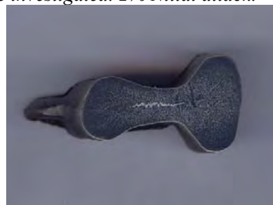
Fig. 5. Specimen code 3- 2% macro Nital attack.
