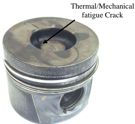
Fig. 5. Engine piston – piston damaged by thermal-mechanical fatigue [10, Minho Univ.].
