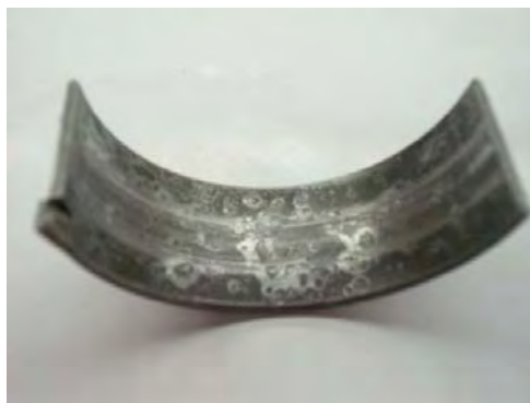
Fig. 14. Journal bearing damaged by abrasion fatigue [Minho Univ.].
