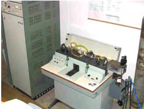
Fig.2. Pulse laser system KVANT 17 (working module, supply and command module and technological module)
