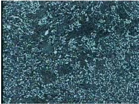
Fig. 6. Optical Micrograph temperature 400 o C, strain rate 0.150 s -1
