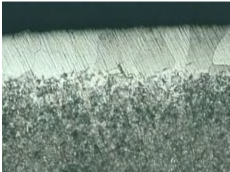
Fig. 7. Nitrocarburized layer on the sample R3 (code R), before of wear process tests.
