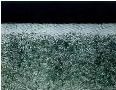
Fig. 8. Nitrocarburized (surface) layer on the sample R2 (code R), before wear process tests.
