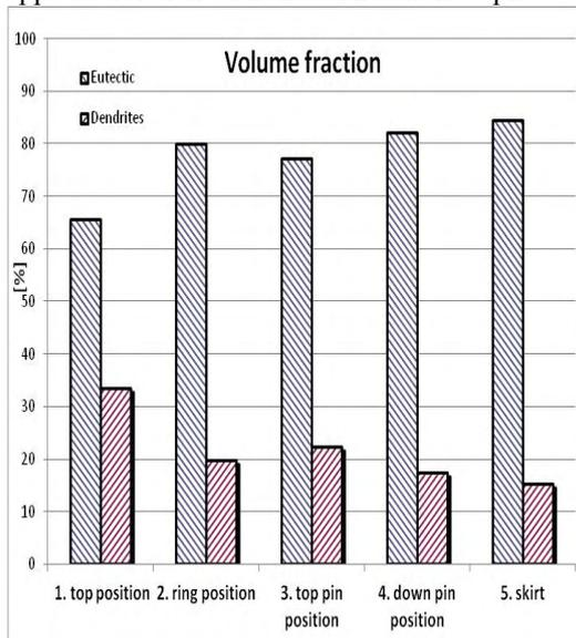
Fig. 4. Volume fraction of eutectic and  $\alpha$ -Al dendrite phase.
