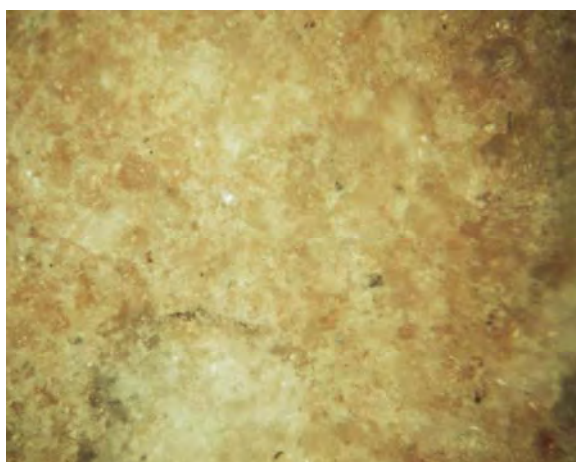
Fig. 4. \delta = 1/2 of refractory wall thickness ( t \approx 700 °C; time = approx. 4 months)
