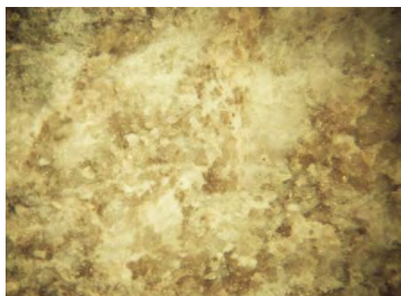
Fig. 3. \delta = 30 mm from the lining – melt metal interface ( t < 1200 °C; time = approx. 4 months)
