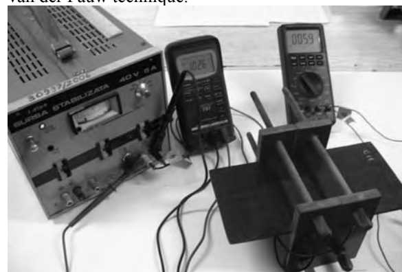
Fig. 2. The experimental arrangement for van der Pauw Technique
