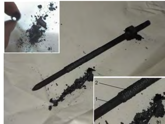
Figure 9. Pyrolysis graphite layer resulted from thermal destruction of polystyrene: a) aspect of the pyrolysis graphite layer resulted from thermal destruction of polystyrene; b) aspect of the deposit of pyrolysis graphite on holder; 1- holder for pyrolysis graphite collection; 2- aspect of the pyrolysis graphite deposit
