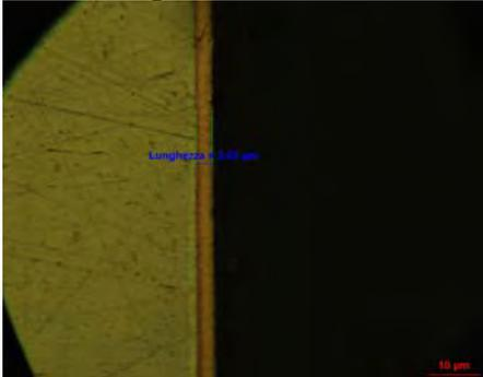
**Fig. 2.** Section from sample TiN-U<sub>0</sub> layer thickness 3.03  $\mu\text{m}$ .
