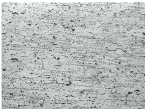
Fig. 11. The microstructure of the Al-Zn alloy after quenching in solution and artificial ageing at 200°C for 3 hours (x100, attack natal).
