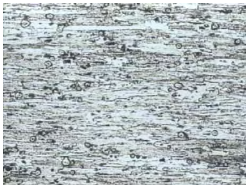
Fig.10. The microstructure of the Al-Zn alloy after quenching in solution and natural ageing (x100, attack natal).
