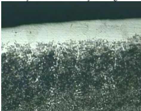
Fig. 8. Nitrocarburized surface layer on the sample R5 (code R), before wear process tests. Treatment: quenching ( t=920^{\circ}\text{C} ) and high tempering ( t=620^{\circ}\text{C} ) followed by water cooling in (dc)continuous current magnetic field and plasma nitrocarburisation at 530^{\circ}\text{C} (7 h) (x100) Nital attack 2%
