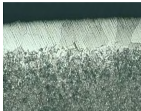
Fig. 9. Nitrocarburized surface layer on the sample R3 (code R), before of wear process tests. Treatment: quenching ( t=920^{\circ}\text{C} ) and high tempering ( t=620^{\circ}\text{C} ) followed by water cooling in (ac) alternative current magnetic field and plasma nitrocarburisation at 530^{\circ}\text{C} (7 h) (x100) Nital attack 2%
