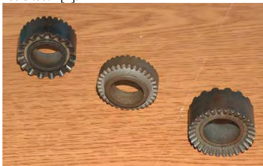
Fig. 5. Sintered satellites from P/M for planetary transmissions.
