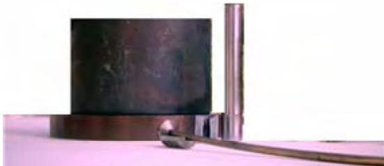
Fig.6. Extrusion die, punch, 3 mm extruded wire
