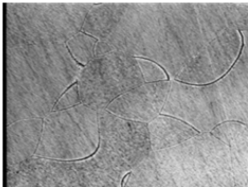
Fig.1. Alloy with 13%Al and 4% Ni, Alloy: Cast aluminium bronze Chemical composition: 13 %Al, 4 Ni, rest Cu Magnification: 50x
