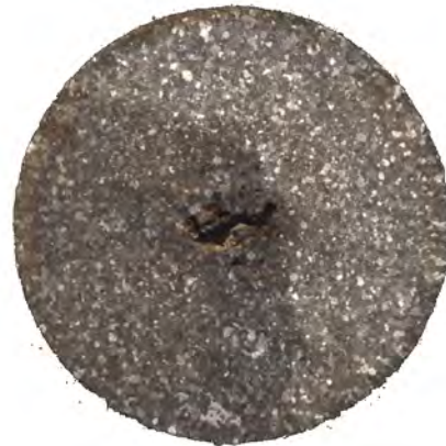
Fig.4. Modified steel macrostructure with 7.07 %Si. It is noticed that the columnar crystals and cracks are not seen.
