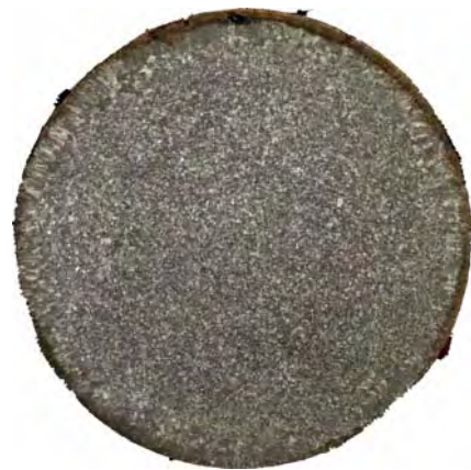
Fig.3. Modified steel macrostructure with 4.48%Si. Columnar crystals are not found
