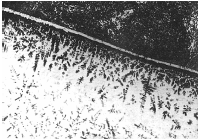
Fig. 6: The dendriform structure of the deposited material in the vicinity of the transition zone.
