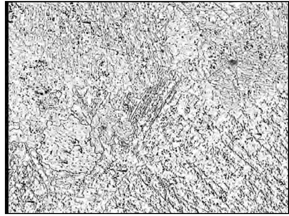
Fig. no. 10. Microstructure of the bath 0,09 % Ni. (x 100). 1% nital attach. Eutectic structure in which fine dispersed particles of Ni-Zn intermettalic compound show up.
