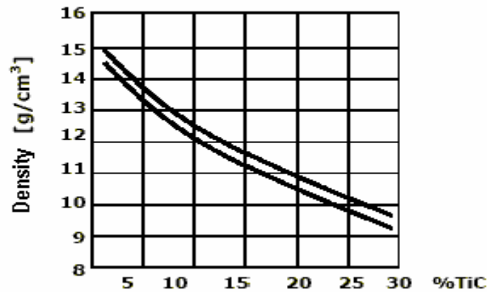
Fig.1 . The dependence of WC-TiC-Co alloy density with the amount of titanium carbide (TiC%)
