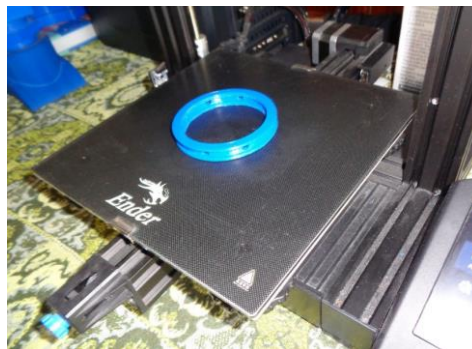
Fig. 7. Lubrication ring landmark, 3D printed using ABS+ filament, on Creality 3D printer, Ender 3 V2
