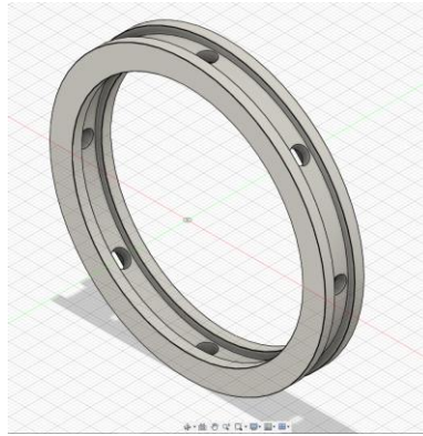
Fig. 3. 3D modeling in the Autodesk Fusion 360 program of the oil ring landmark, resulting in the STL format file for "slicing" before its 3D printing
