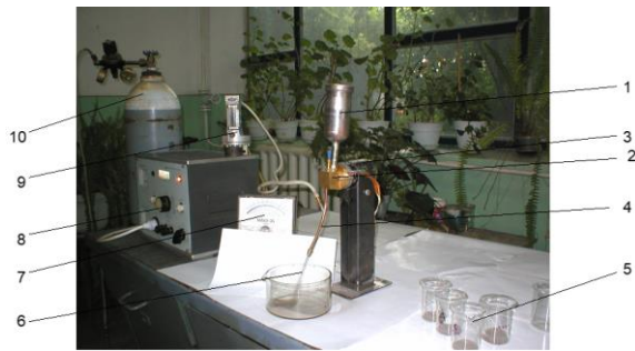
Fig. 2. The test and calibration stand of the injection system: 1 – tank; 2 – dispenser; 3 – direct current electric motor; 4 – directing element; 5 – laboratory beakers; 6 – powder jet; 7 – voltammeter; 8 – autotransformer; 9 – rotameter; 10 – argon cylinder
