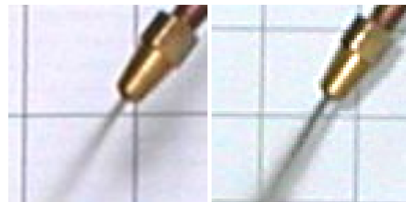
Fig. 3. Aspects of the powder jet generated at different supply voltages and argon flow rates
