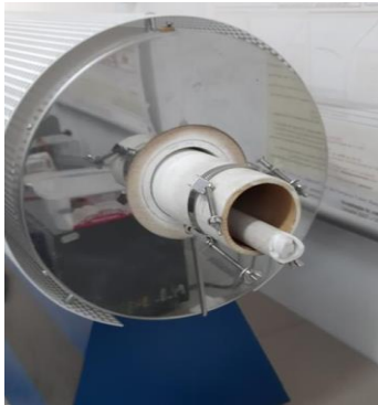
Fig. 5. The furnace LENTON used for sintering
