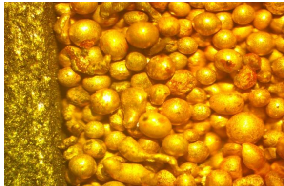
Fig. 3. The graphite mould with the powder that was ready to be sintered
