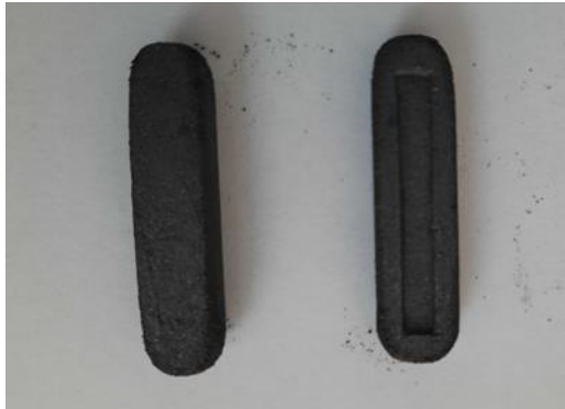
Fig. 2. The mould with the two semi-cylindrical components used for the free casting of CuSn12 powder samples
