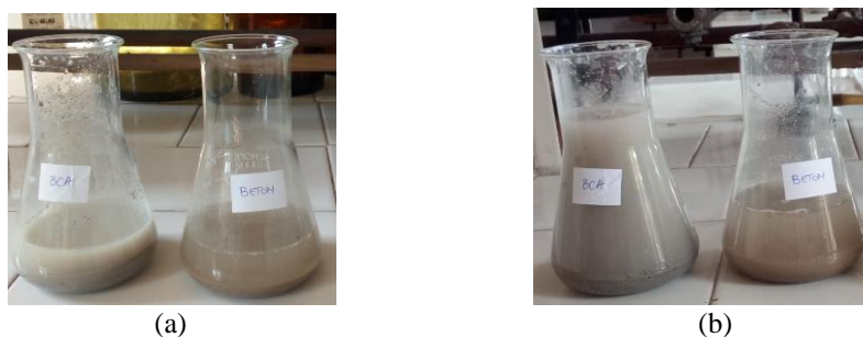
Fig. 6. The construction materials in contact at L/S = 2+8 L/kg: (a) for 6 hours; (b) for 18 hours
