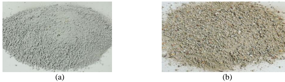
Fig. 4. The test granular material with d < 40 mm: (a) Autoclaved Aerated Concrete AAC; (b) Concrete
