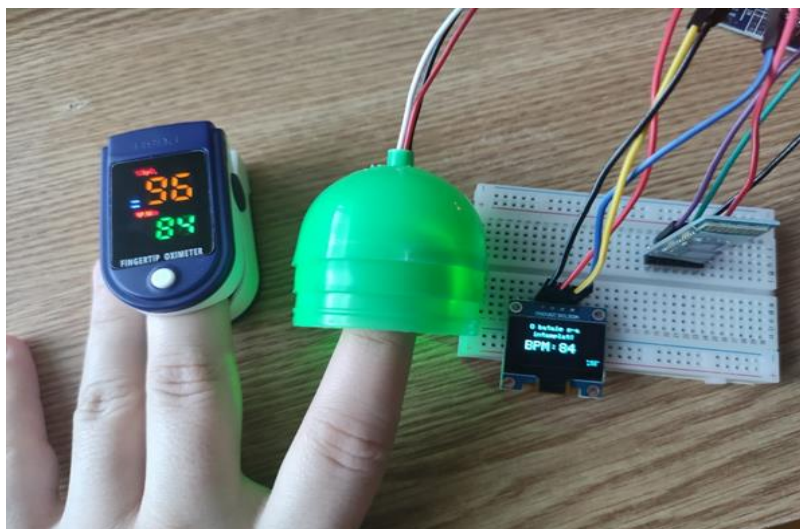
Fig. 7. The results validation for the heart rate system proposed using a pulse oximeter
