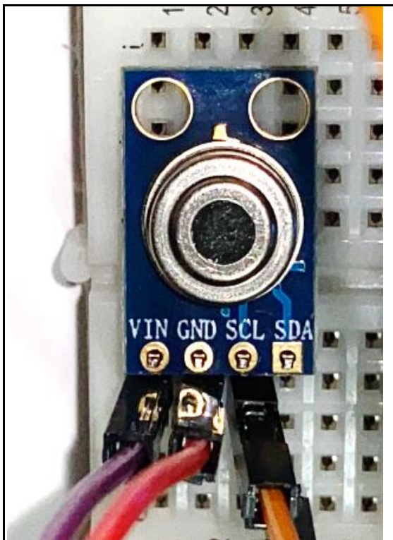
Fig. 2. The MLX90614 sensor pin connections
