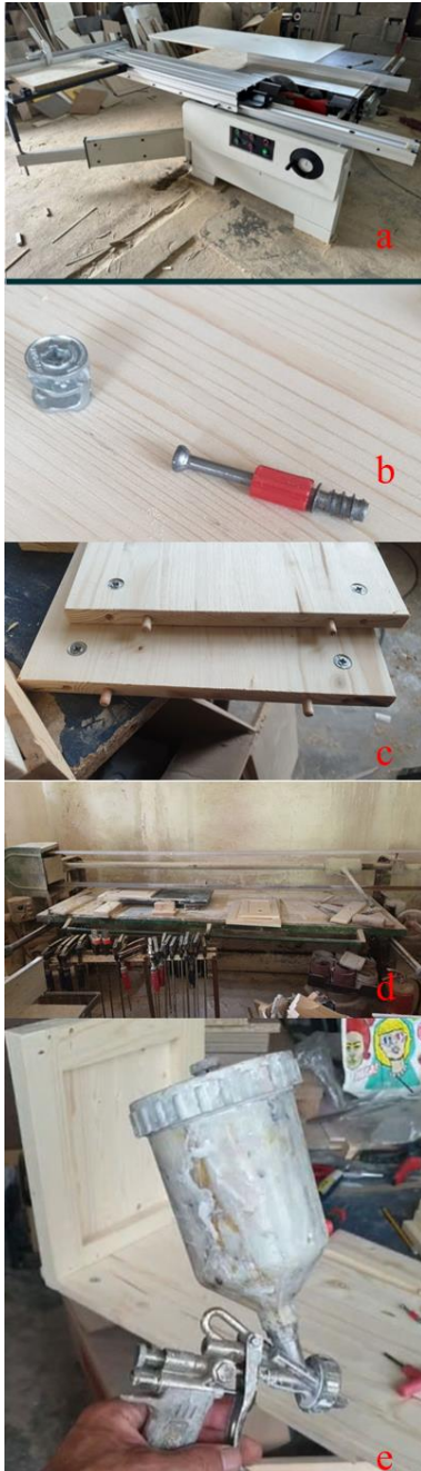
Fig. 5. Processing stages of the wooden amplifier case: a. Circular saw for material cutting; b. Eccentric cam for fastening; c. Wood dowels for fastening; d. Belt sander; e. Spray gun
