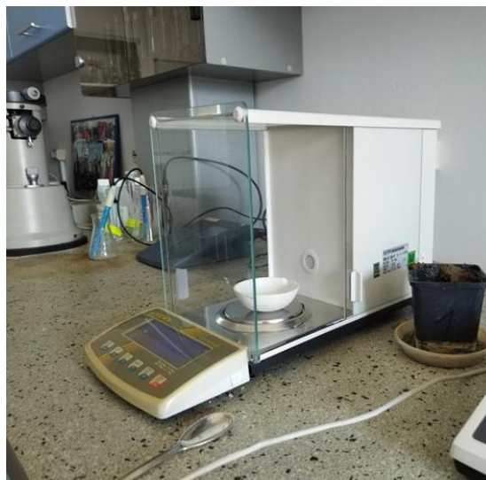
Fig. 1. Weighing the soil sample
