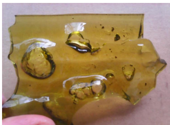
Fig. 3. Superficial cracks on the surface of the part
