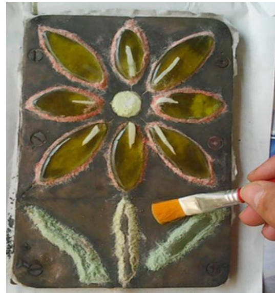
Fig. 11. Preparation of the plate-inlay assembly for thermoforming
