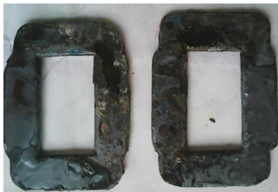
Fig. 1. Metal frames used for the study of glass embedding inside them
