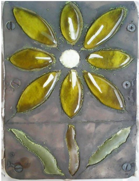
Fig. 12. Decorative object made by inlaying glass in metal (stainless steel) through thermoforming
