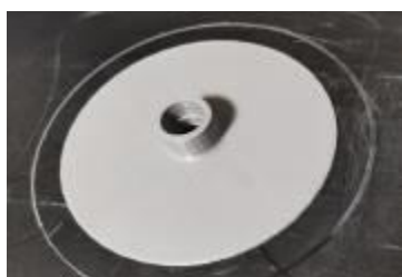
Fig. 12. 3D-printed large gear blank for the extrusion drive assembly
