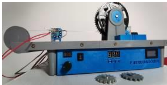
Fig. 15. The extruder system assembled view
