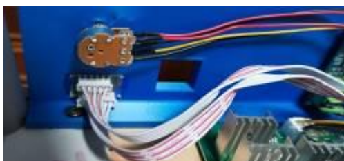
Fig. 13. The display interface and switch installed
