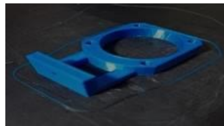
Fig. 10. The ventilation fan support 3D printed
