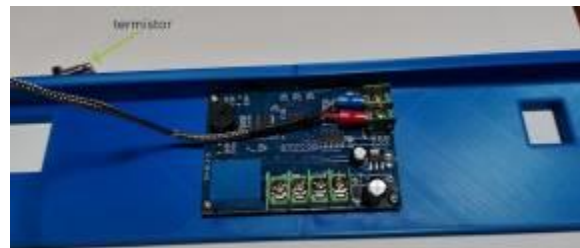
Fig. 4. The front panel with thermostat module installed
