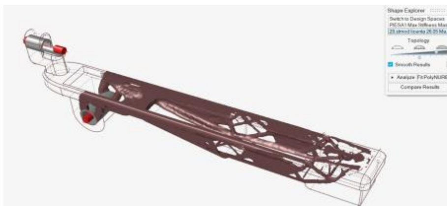
Fig. 4. Top view of the optimized structure showing material distribution
