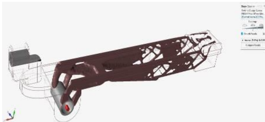
Fig. 3. Topologically optimized 3D model
