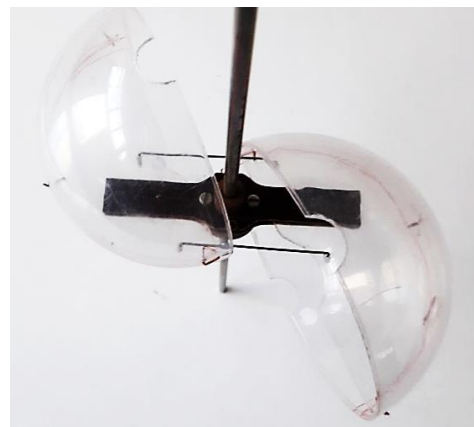
Fig. 5. Experimental Model for VAWT with hemispheric cups
