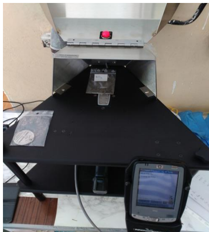
Fig. 5. Dry sludge sample, inserted into the X-ray spectrometer
