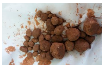
Fig. 5. Mixture of dried pellets obtained with different binders
