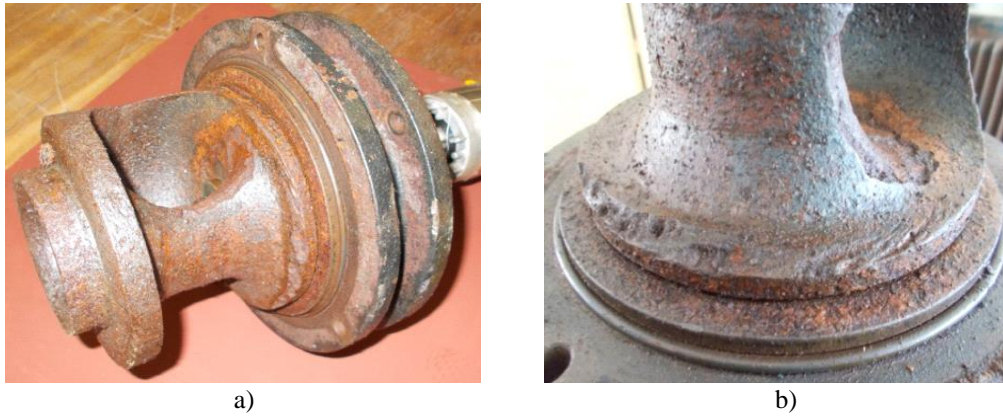
Fig. 7. Single-channel low pressure centrifugal pump; a) a rotor; b) rotor corroded and worn area
