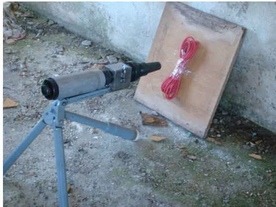
Disrupter ready for shooting. The distance between the detonator wick and the disrupter is 10 cm
