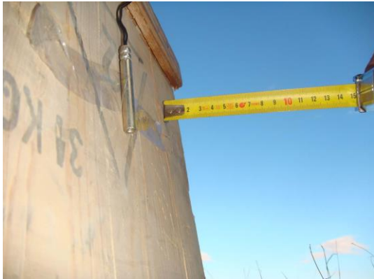
The distance between the electrically detonating cap and the disruptor is about 15 cm
