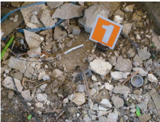
The electrically detonating cap is deformed after the disruption
