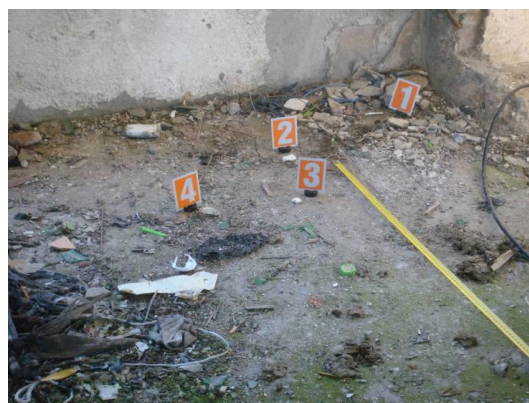
The distance of approx. 280 cm at which fragments of plastic explosive were projected after disruption
