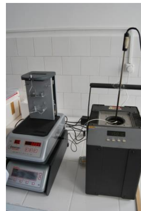
Fig. 7. Calibration thermobalance sensor at 15°, 20° and 30 °C
