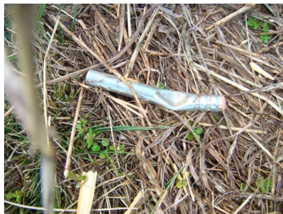
Electrically detonating cap deformed after disruption
