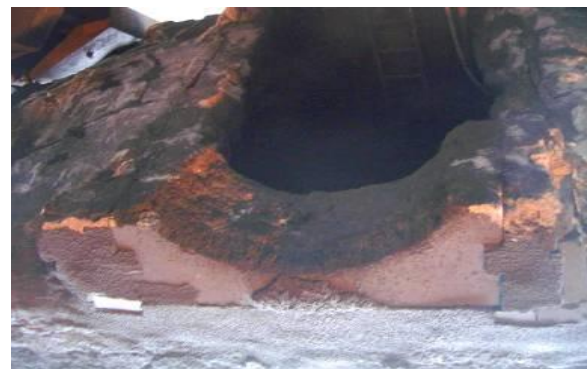
Fig. 6. Charging hole (mouth) 300T casting ladle after 1020
