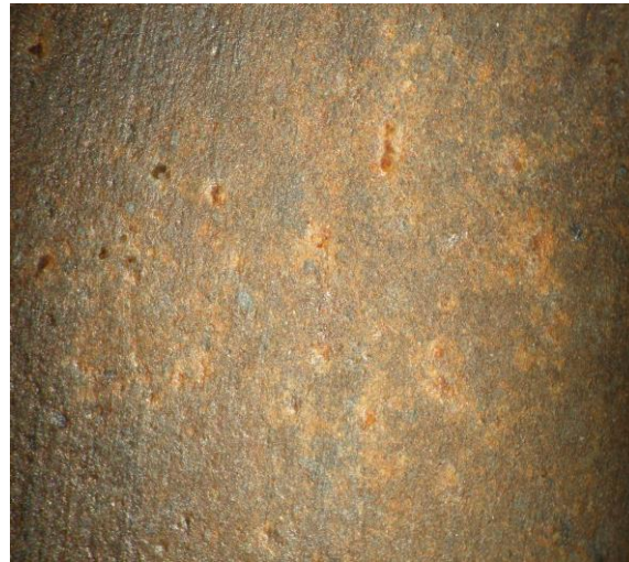
Fig. 12. Surface appearance of uncoated NbC samples after corrosion
