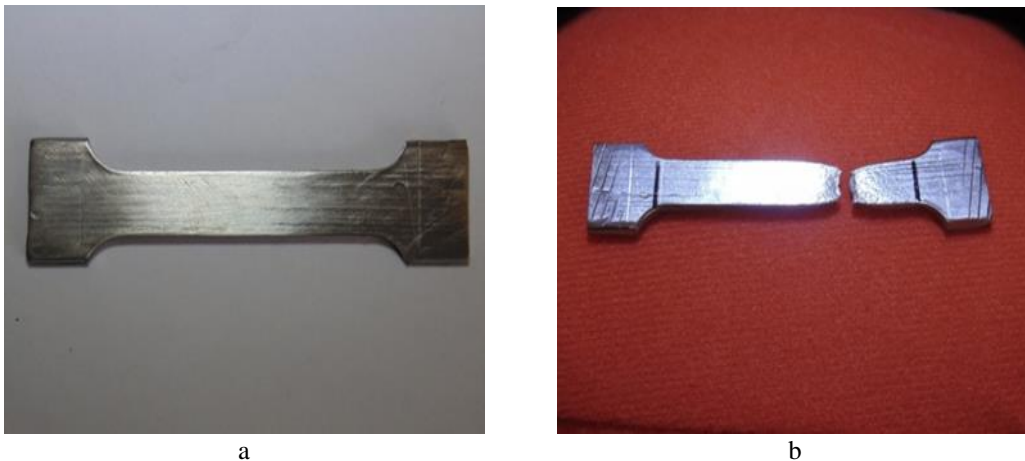
Fig. 3. Standard test specimen of alloy Ti10Zr tensile testing: before (a) and after the test (b)
