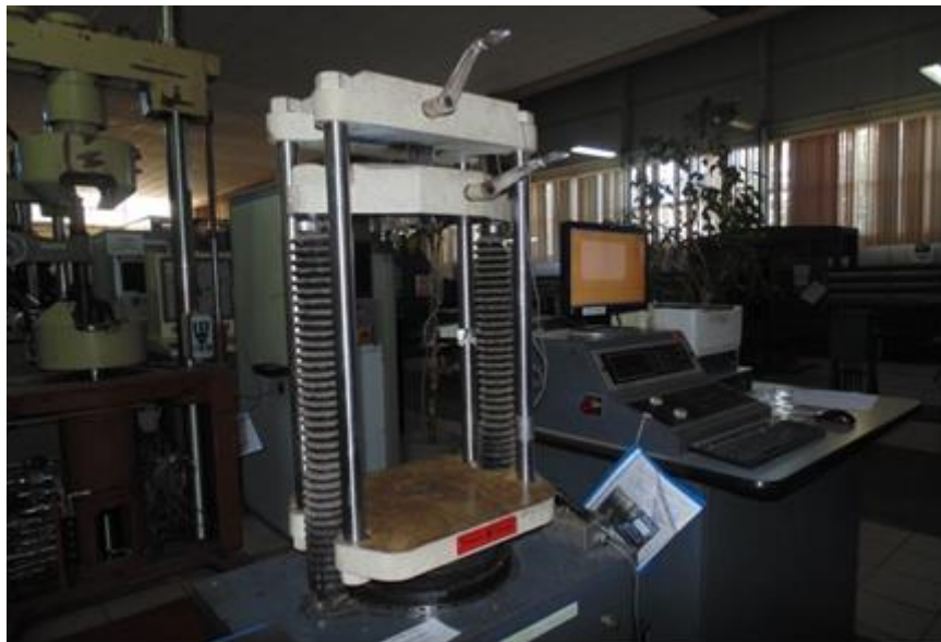
Fig. 4. Tensile test machine to determine the mechanical properties of the alloy Ti10Zr (making the specimen from the initial blank and the tensile test)
