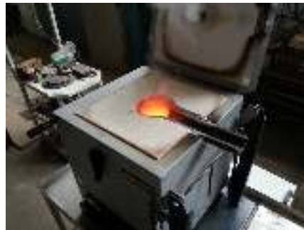
Fig. 2. Electric crucible furnace for copper wire scrap melting
