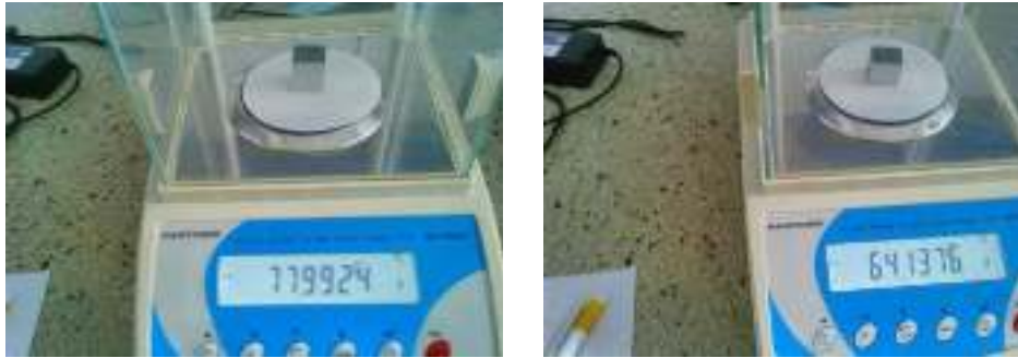
Fig. 2. Weighing samples subjected to the corrosion test
