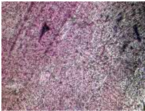
Fig. 3. Microstructure of the Cu – Sn powder, attacked by ferric chloride reagent
