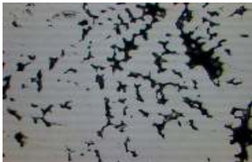
Fig. 6. Microscopic appearance (optical microscopy without metallographic attack, magnification X100) of the Co-Cr alloy samples (ADORON LX40626), Samples from metal crown [5]
