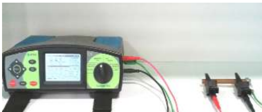
Fig. 5. Electric insulation resistance measurements
