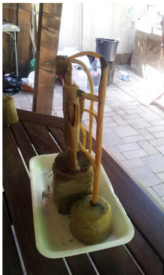
Fig. 6. Casting network for the casting of the "Knight IV"
