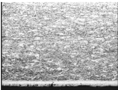
Fig. 4. Microstructure, sample 2: (CN650 °C/80 min + O, 100x)
