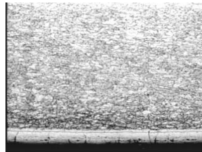
Fig. 6. Microstructure, sample 4: (CN650 °C/120 min + O, 100x)
