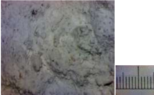
Fig. 8. Macrostructure of the KERMAG LTD90 sample before casting (calibration 63x stereomicroscope)
