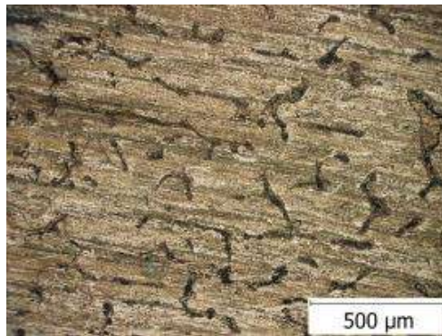
Fig. 6. Spots of burned emulsion with atypical forms
