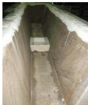
Fig. 7. Tundish with Tundex 160 AS after drying
