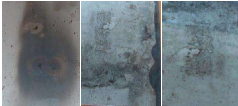
Fig. 3. Burned emulsion on the surface of the heat treated strip (x1/10)
