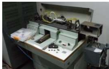
Fig. 2. YAG laser system image: pulsed Nd (KVANT 17)
