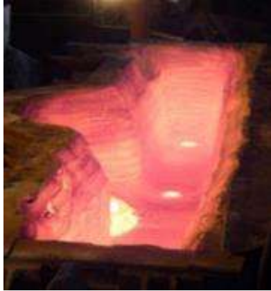
Fig. 5. Tundish gunited after drying
