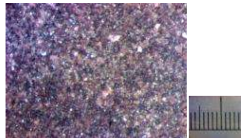
Fig. 12. Macrostructure of the TUNDEX 160 AS sample before casting (calibration 63x stereomicroscope)
