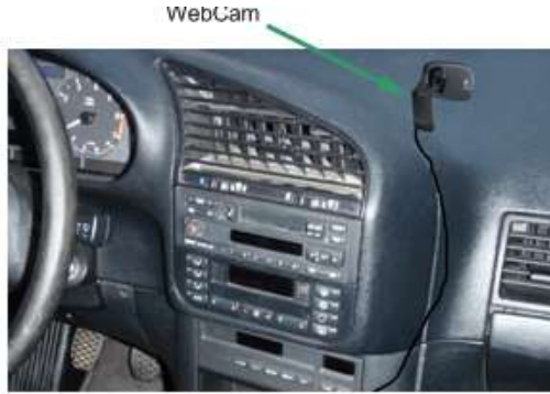
Fig. 3. Positioning of the web camera on dashboard
