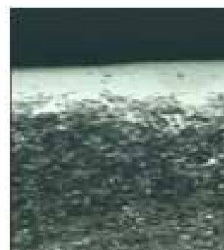
Fig. 9. Superficial layer thickness before wear tests, for T14 treatment regime (x100) (with d.c. magnetic field regime)
