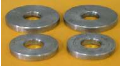
Fig. 2. Couples of rollers corresponding to different sliding degrees \zeta [6, 8]
