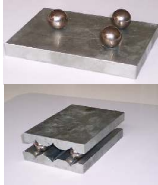
Fig. 5. (a, b) Details on the rolling-contact elements: a) the set of 3 identical balls; b) the whole rolling couple
