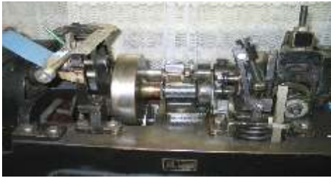
Fig. 3. Wear tests were carried out on an Amsler machine [6, 8]
