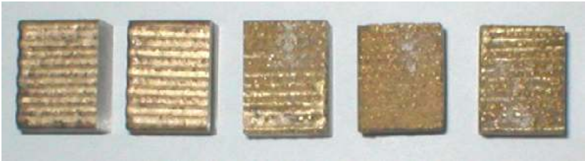
Fig. 2. Surface of samples clad by thick layers of aluminum bronze
