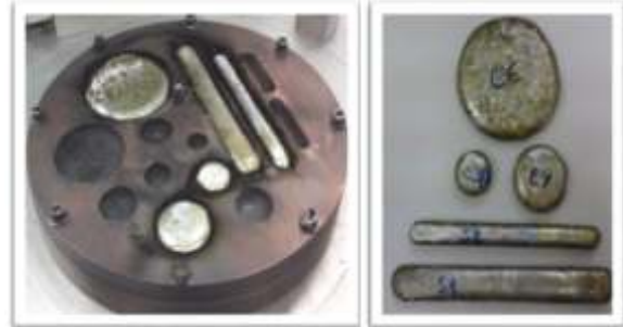
Fig. 5. Commercial Co-Cr-Mo alloy after solidification – casting samples
