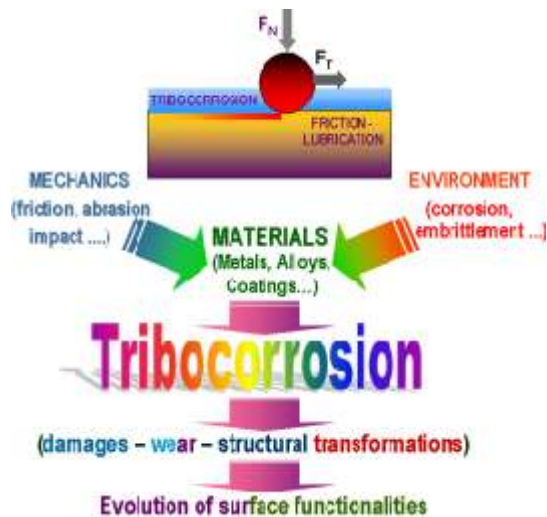
Fig. 2. Synergy of friction and corrosion processes occurring simultaneously on the surface of a material
