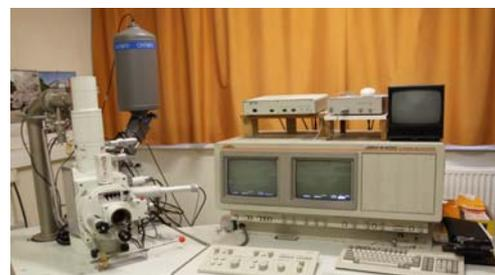
**Fig. 5.** System EBSD - Microscope JSM-6400
