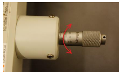
Fig. 7. The micrometric screw of the Variable Attenuator
