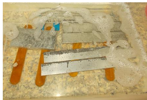
Fig. 2. Place the samples in the vessel with the corrosion solution
