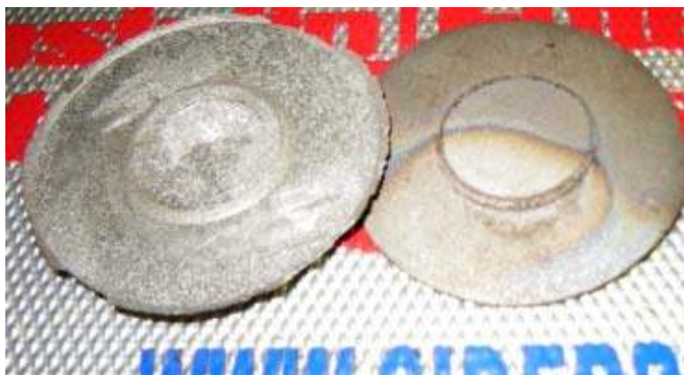
Fig. 6. Coatings detached; left - with bonding layer deposition; right - without bonding layer deposition
