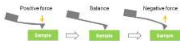
Fig. 9. Schematic of AFM tip/specimen contact under negative and positive applied loads [11]
