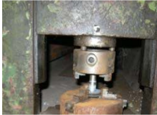
Fig. 4. Normal adhesion strength testing
